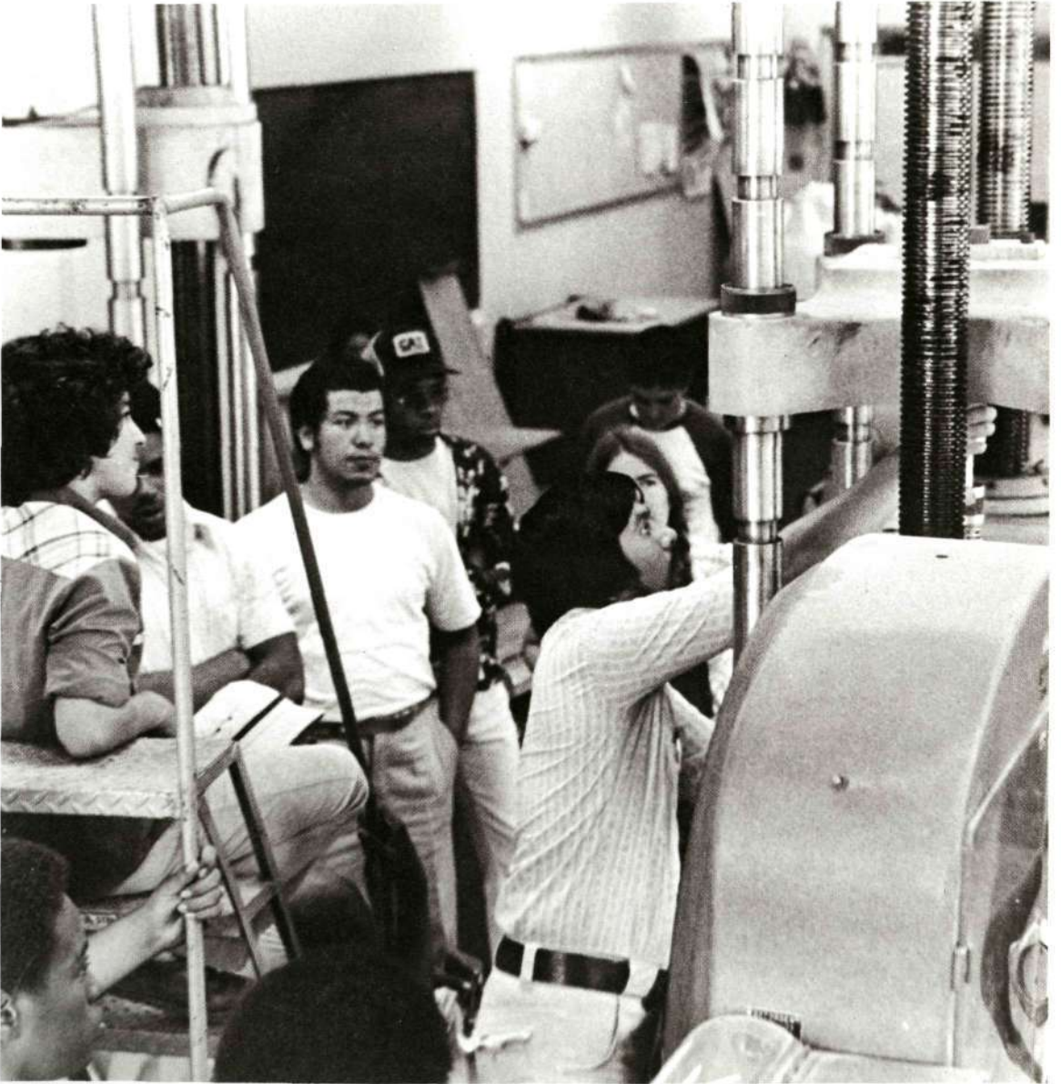
Students in the Mathematics, Engineering, Science Achievement (MESA) program at California State University, Long Beach, learn to use a hydraulic universal testing machine to measure stress-strain relationships in standard tensile specimens.
